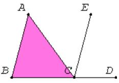
Let ABC be the triangle. Extend BC, and draw CE parallel to AB. That's the construction in the previous proposition I.31. Then by I.29, angle B equals angle ECD, and angle A equals angle ACE. Thus the interior angles of the triangle sum to angle CBA plus angle ECD plus angle ACE. But that's a straight angle, the sum of two right angles.
