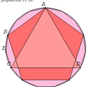
Here's what Euclid did. Construct the equilateral triangle and the regular pentagon in the circle. Let AC be one side of the triangle and AB one side of the pentagon. Bisect the arc BC at E. Then BE and EC are two adjacent sides for the 15-gon. Just repeatedly cut off arcs of that size from the circle to get the rest of the 13 sides.
