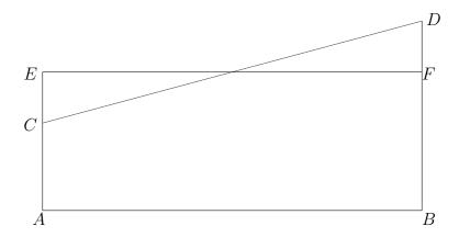
But the area of this trapezoid ABDC is the same as the area of a rectangle ABFE on the same base but whose height AE = BF is the average height of the left and right sides of the trapezoid. Thus the distance traveled under constant acceleration is the same as the distance traveled by an object going a constant velocity, that being the average of the initial and final velocities.
