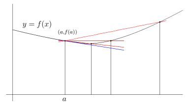
As b approaches a, the red secant lines get closer to the curve y = f(x) near x = a, that is, they approach the blue tangent line at x = a. Unlike the secant lines, the tangent line doesn't cross the curve but only touches it. The word "tangent" comes from the Latin *tangentem* for "a touching." It's been used in mathematics since 1583.
